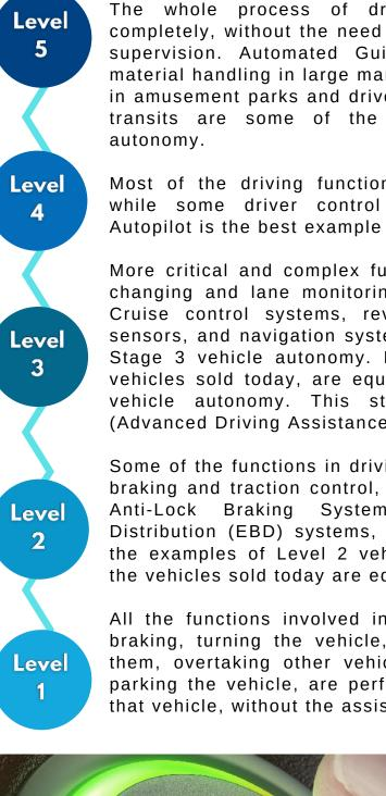
The whole process of driving a vehicle is automated completely, without the need for any human input, control and supervision. Automated Guided Vehicles (AGVs) used for material handling in large manufacturing plants, roller coasters in amusement parks and driverless metro trains used in public transits are some of the examples of Level 5 vehicle autonomy.
